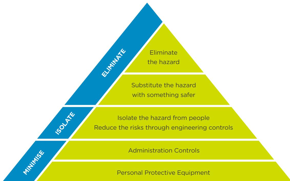
Figure 1: Hierarchy of controls
